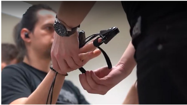
FIGURE 11. Placement of EDA electrodes on the participant's hand.
