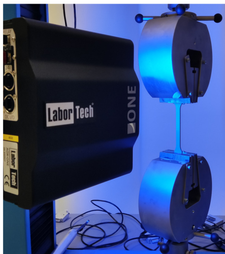
Figure 5. Hardware configuration according to ISO 527 standard.
