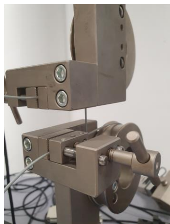
Figure 6. Hardware configuration for measuring filaments.
