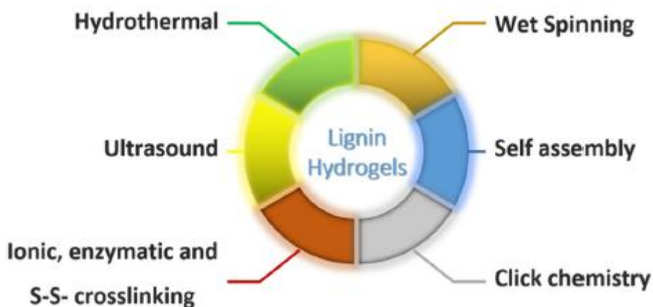
Fig. 5. Schematic representation of the strategies for the synthesis of lignin-based hydrogels.
