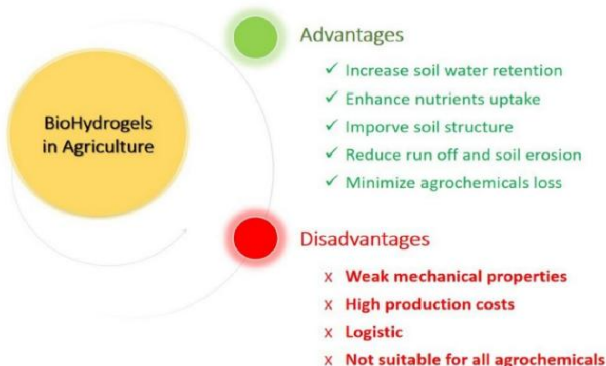
Fig. 4. Disadvantages and advantages of biopolymeric hydrogels in agriculture. Reconstructed from Tariq et al. [48]. WHC = water holding capacity.
