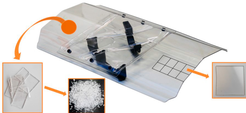
Fig. 2. The preparation process of test plates and grits from polycarbonate shield.
