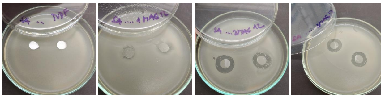
Figure 4 The inhibition zones of S. aureus (SA) nanofibrous membranes without/with added MAG C12 (from left to right: 0 wt.%, 1 wt.%, 2 wt.%, 3 wt.%)
