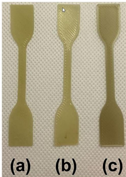
Fig. 8. 3D printed specimens formed from filaments based on (a) P3HB-co-4HB (M1), (b) P3HB-co-4HB with 2 wt% of citrofol BII (M3) and (c) blend of P3HB-co-4HB/PLA 50/50 with 2 wt% of citrofol BII (M4).
