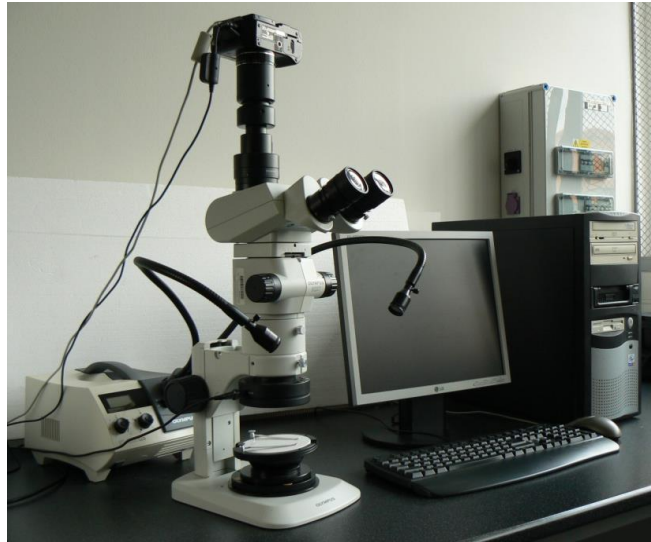
Fig. 6. Configuration of the microscope Olympus SZX7
