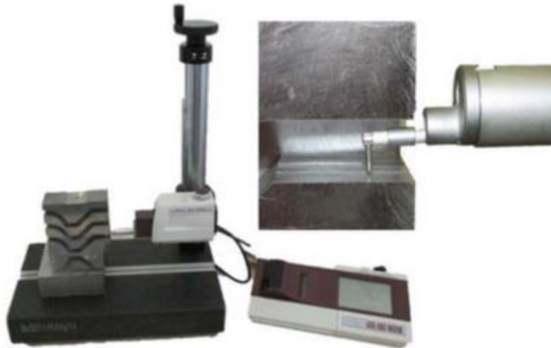
Fig. 9 Surface roughness measurement device Mitutoyo with detail of the tip
