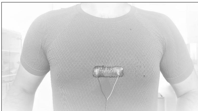
**Figure 7.** Sensor based of MWCNT (KMnO<sub>4</sub>) fixed on a sports T-shirt for practical application of a human breath monitoring.
