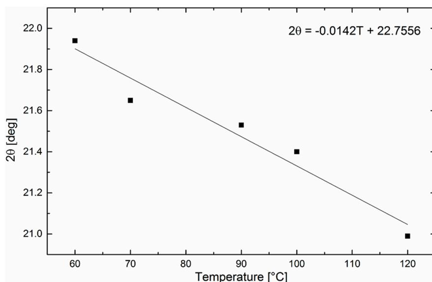
**Figure 4.** Position of an amorphous halo as a function of the temperature of melted PEO.
