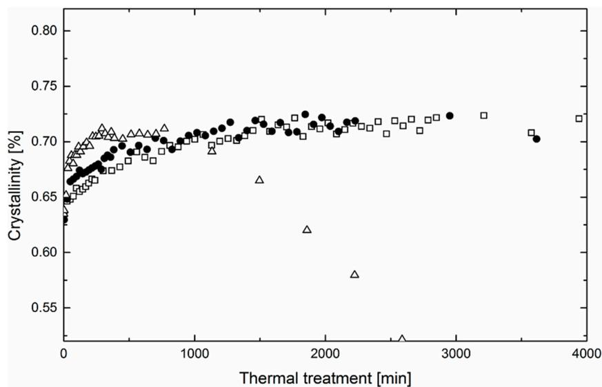
**Figure 5.** Evolution of crystalline structure of nanofibrous webs prepared from water/PEO solution at three different temperatures in time (squares denote 40 °C, circles 50 °C, and triangles 60 °C).
