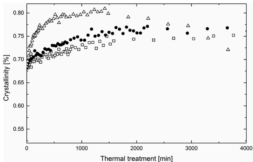
**Figure 6.** Evolution of crystalline structure of nanofibrous webs prepared from methanol/PEO solution at three different temperatures in time (squares denote 40 °C, circles 50 °C, and triangles 60 °C).
