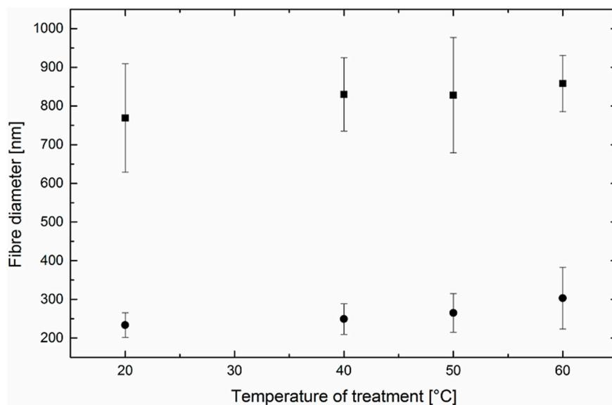
**Figure 2.** Effect of temperature on the diameter of fibers obtained from PEO solutions. Square symbols denote methanol solutions and circles denote water solutions.
