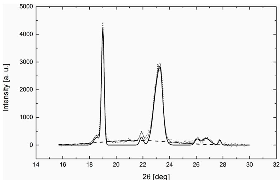
**Figure 3.** Diffractogram of nanofibrous PEO sample separated into individual crystalline peaks (solid thick line) and an amorphous halo (dashed line). The dotted line shows the experimental data and the solid thin line represents the amorphous and crystalline part fitted together.
