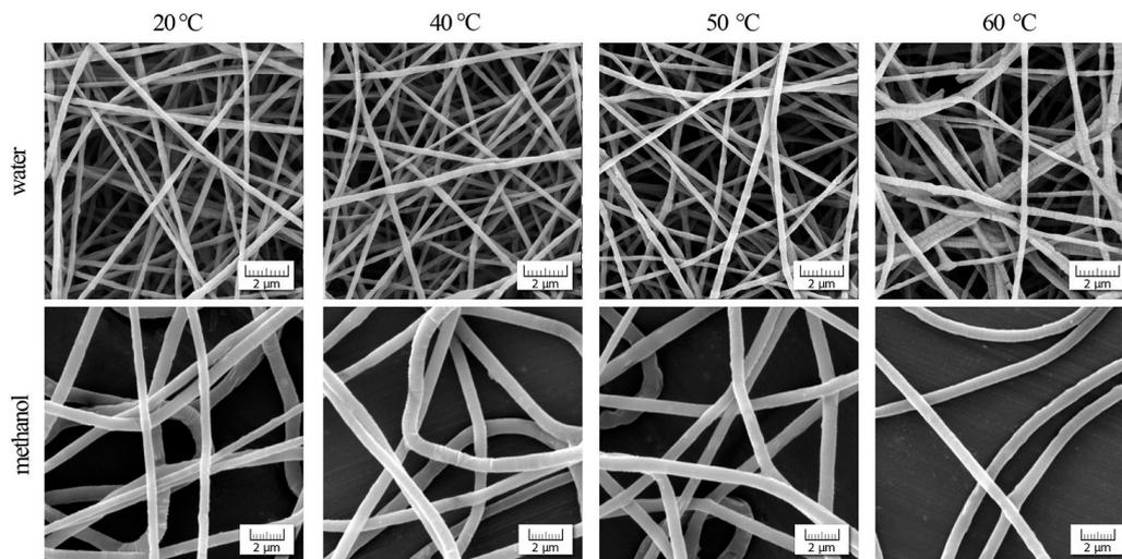
**Figure 1.** Effect of temperature on morphology of fibers obtained from PEO solutions.
