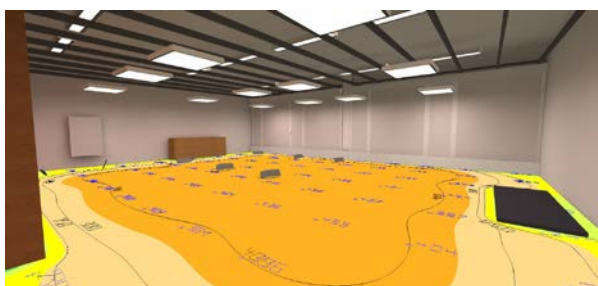
Fig. 7. Example of the illuminance distribution on a work plane throughout the lab.
