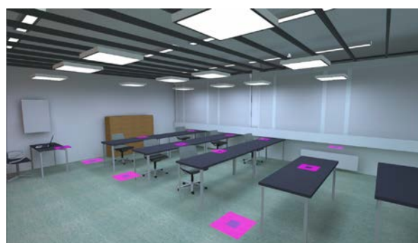
Fig. 3. Model of the light laboratory in 3D with the observation points.
