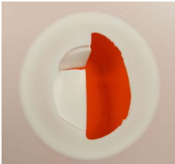
Fig. 7. HIPS deformation after drop weight test at 150 J.
