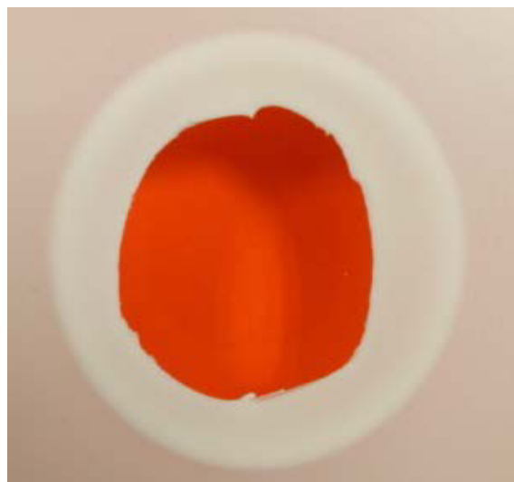
Fig. 8. HIPS deformation after drop weight test at 200 J.
