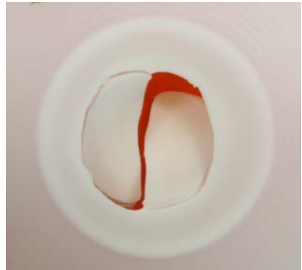
Fig. 4. HIPS deformation after drop weight test at 30 J.
