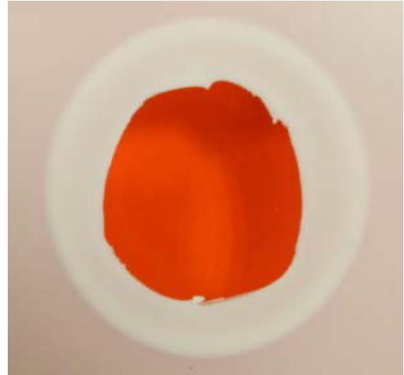
Fig. 9. HIPS deformation after drop weight test at 230 J.
