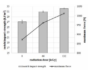
**Fig. 9.** Notch impact strength and maximum force (PA 7T GF 56, test temperature -75 °C).
