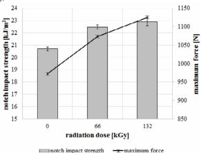
**Fig. 8.** Notch impact strength and maximum force (PA 7T GF 56, test temperature -50 °C).
