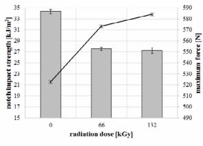
**Fig. 4.** Notch impact strength and maximum force (PA 66 GF 30, test temperature – 100 °C).
