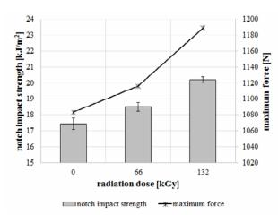
**Fig. 7.** Notch impact strength and maximum force (PA 7T GF 56, test temperature -23 °C).
