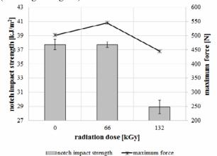
Fig. 12. Notch impact strength and maximum force (PA 7T GF 56, test temperature -150 °C).
