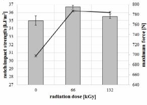
Fig. 10. Notch impact strength and maximum force (PA 7T GF 56, test temperature -100 °C).
