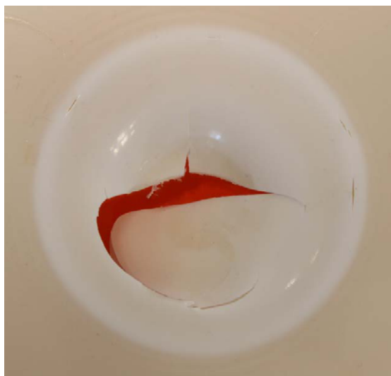
Fig. 8. ABS deformation after drop weight test at 100 J after climate test (up view).
