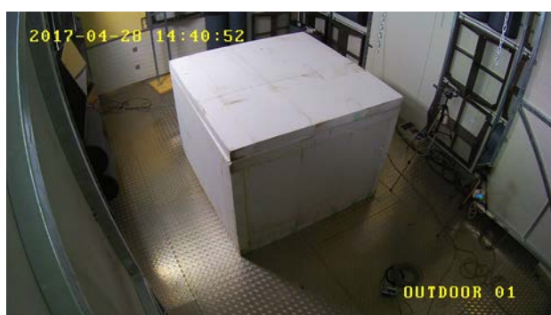
Figure 2 Testing box inside the calorimetric chamber
