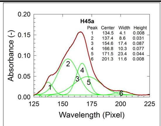
**Figure 3.** NIR spectrum of Dark 45 % chocolate and its components.
