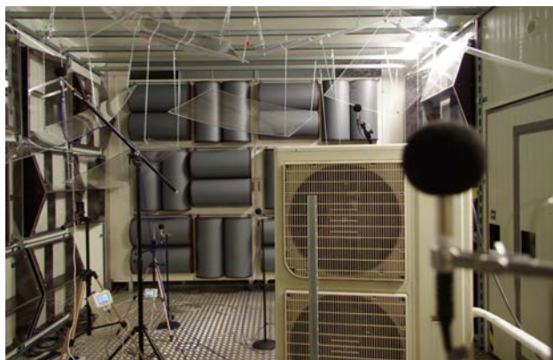
Figure 1. Reverberation chamber at FAI UTB in Zlín, CZ.
