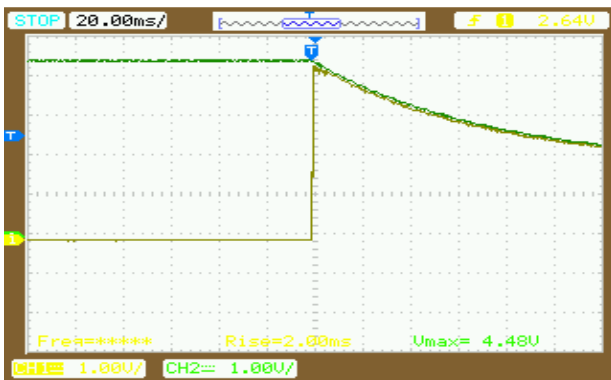
Fig. 4 the output of the device with TEC 12708
