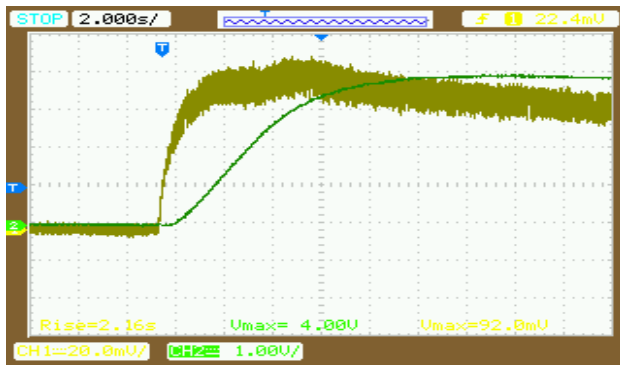
Fig. 8 the output with 47k \Omega load and TEC MCHPE 127-10-08-E
