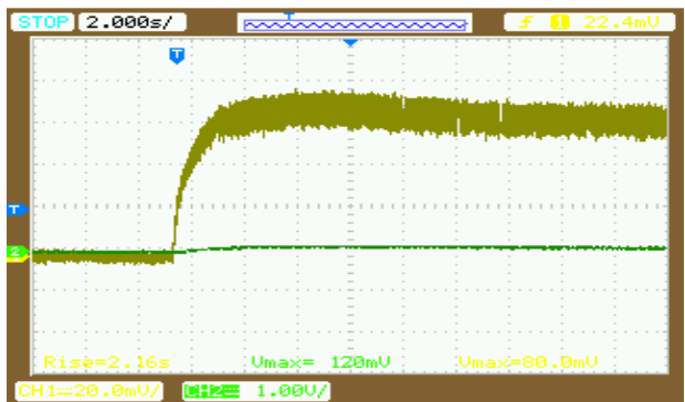
Fig. 9 the output sequencing with load 1k \Omega and TEC RC 12-4
