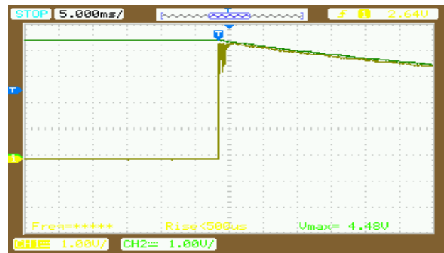
Fig. 5 the output of the device with TEC MCHPE-127-10-08-E
