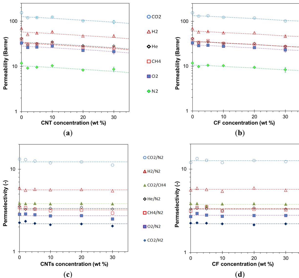
The applicability of the Maxwell model is interesting because ideally it applies to systems containing low concentrations of spherical fillers. In all cases, the gas transport behavior of the CF-filled membranes is practically identical to that of the CNT-filled membranes. Therefore, only the
