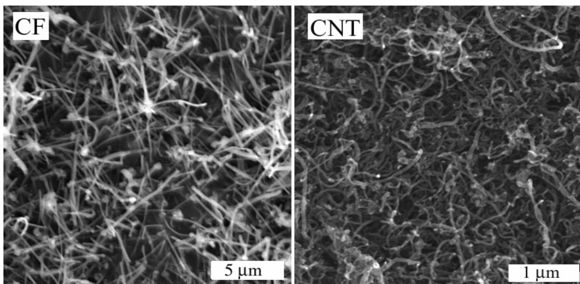
**Figure 2.** SEM images of fractured surface of EOC/CF composites (20 wt % CF) and EOC/CNT composites (25 wt % CNT).
