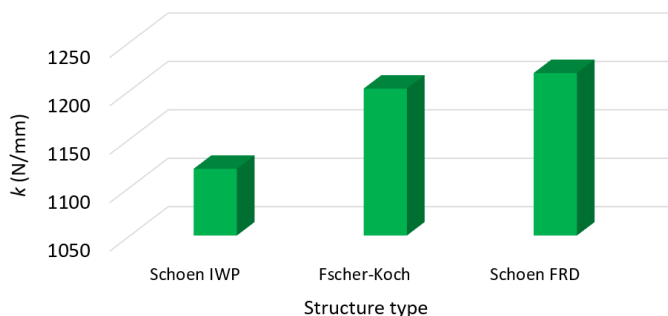
Fig. 4 Stiffness in bending of the individual types of structures.
