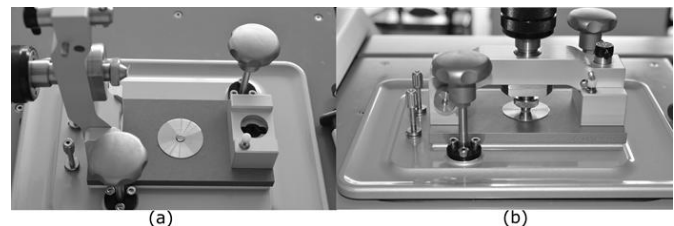
Fig. 2. Measurement setup. (a) ATR silicon crystal with PSS applied. (b) Hemostat sample applied and fixed.
