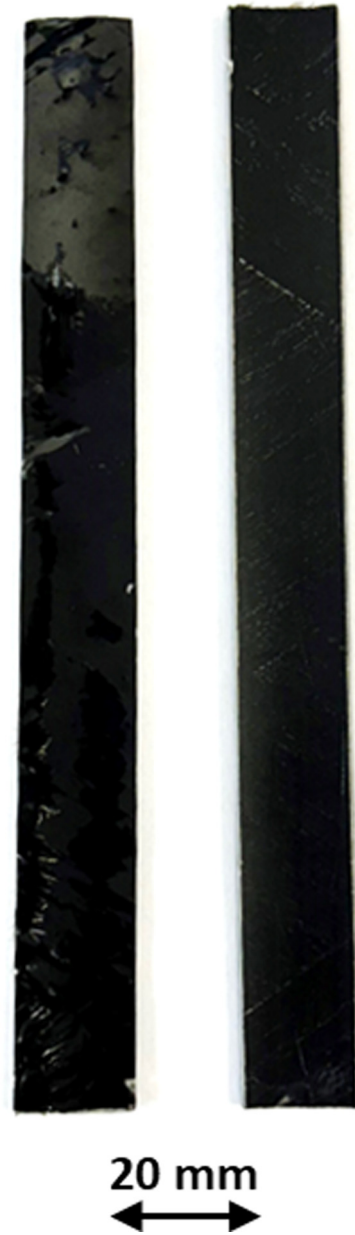
Figure 1: Photograph of cutouts of tested composite pipes.
