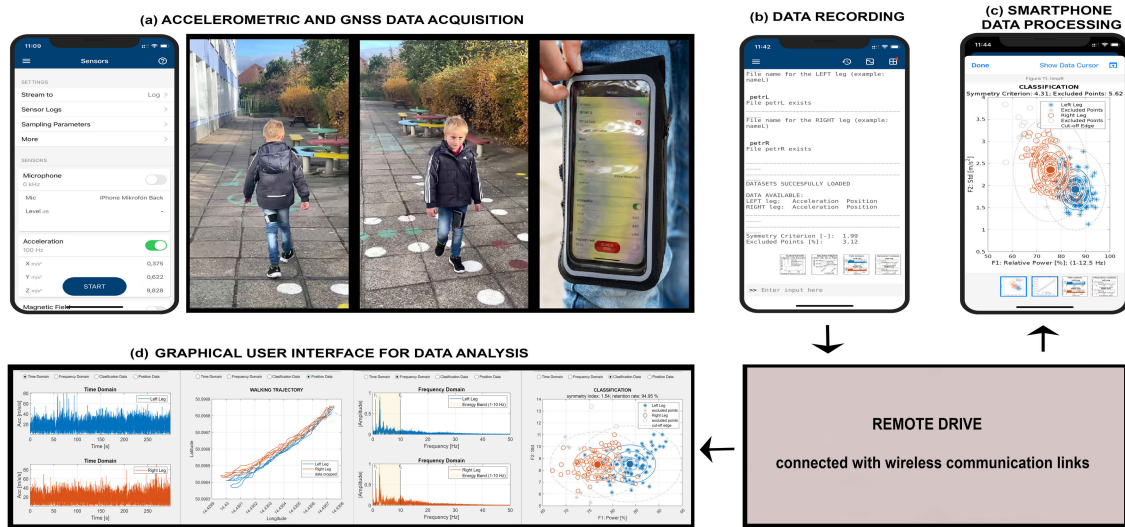
FIGURE 1. Principle of motion data acquisition during walking tests presenting: (a) initialization of sensors and conducting a walking experiment with the recording of accelerometric and GNSS positioning data, (b) the use of mobile Matlab on a smartphone for data recording and wireless export to a remote drive, (c) evaluation of the symmetry coefficient on the smartphone using the remote drive, and (d) a graphical user interface for detailed data analysis, which allows for the presentation of time-domain accelerometric data, a GNSS record of walk positioning, evaluation of gait frequency components, and the distribution of gait features evaluated separately from the left and right legs using data stored on the remote drive.
