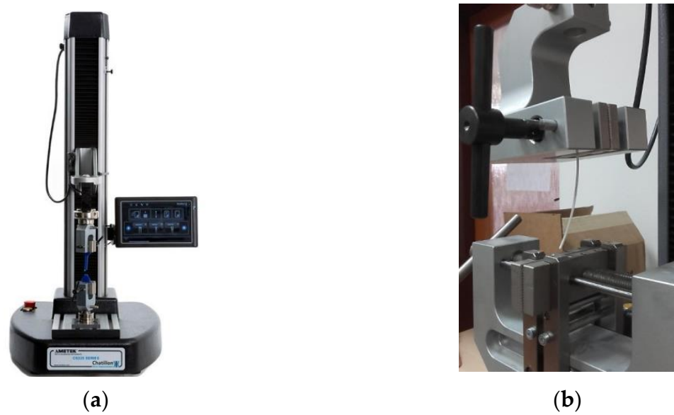
Figure 5. The preliminary tests of White EasyABS filament properties: (a) desktop tensile testing machine CS 225; (b) testing set.
