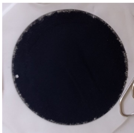
Figure 1. Free-standing film of MXenes prepared by VAF on a Celgard membrane ( \varnothing = 4 cm, h = 18 \mu m).
