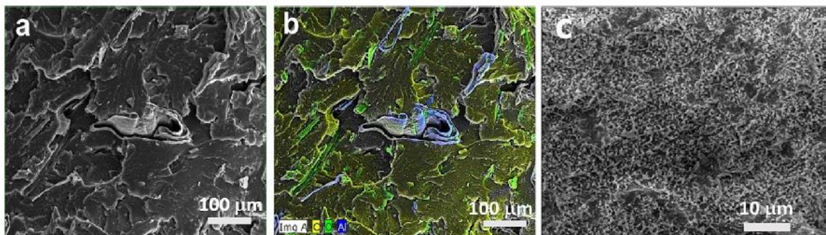
Fig. 2. a) SEM image of TP , b) EDS mapping of TP , c) TP/PW = 60/40 w/w.
