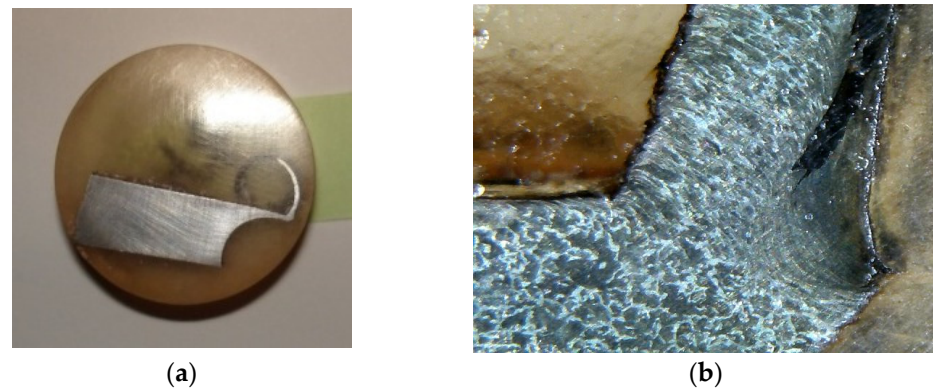
Figure 5. Investigated sample of a chip, (a) ground and polished, (b) etched, magnified 200×.
