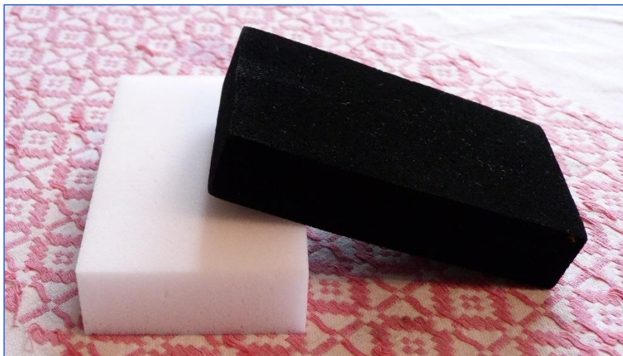
Figure 1. Melamine sponge (a) before (left) and (b) after the deposition of polypyrrole in the presence of silicotungstic acid (right).
