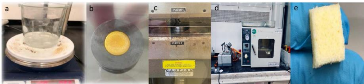
Fig. 1. a.) Mixing of components, b.) casting into the form, c.) crosslinking/foaming, d.) cleaning in an oven, e.) Qwax foam.
