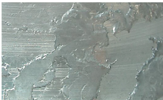
Fig. 1. Fatigue cracking caused by dynamic load.
