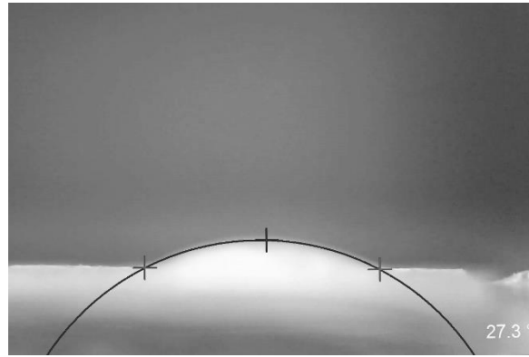
Fig. 5 Contact angle measurement for PU918 (water drop)
