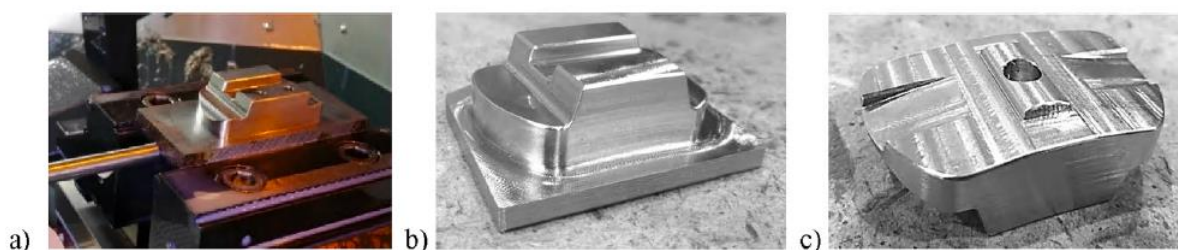
Fig. 12. (a) Process of the lever machining; (b) the lever after machining from one side; (c) machined lever.
