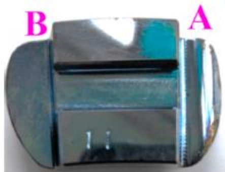
Fig. 27. A lever treated by electroless nickel plating before test.
