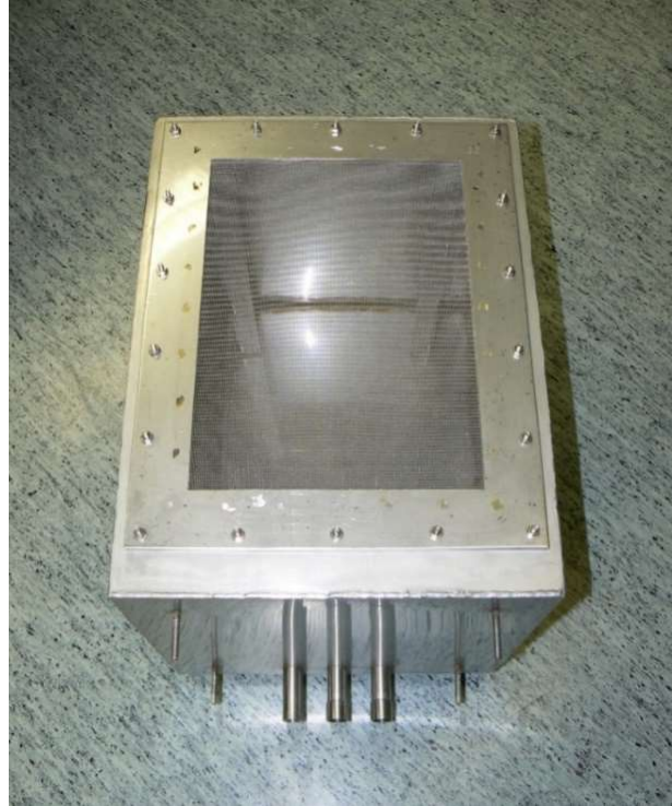
Fig.2. Shielding enclosure for a security camera.
