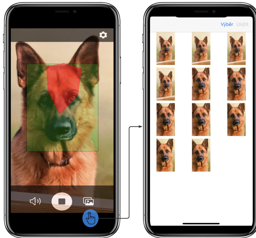
Figure 3: Two main application's screens: automatic shooting screen (on the left) and display of automatically photographed photos (on the right). The shooting screen shows the detected dog face rectangle in green and the identified dogface landmarks in red.
