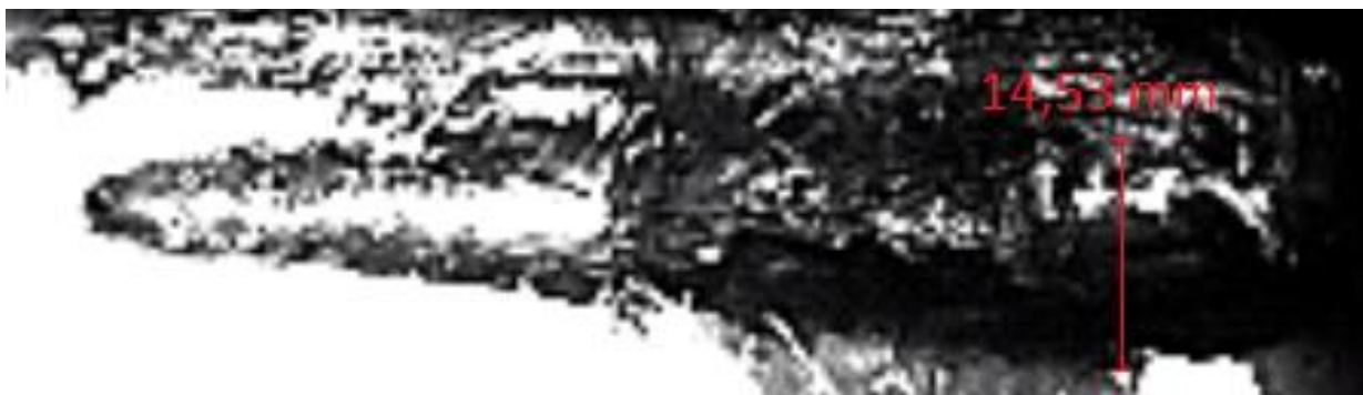
Fig. 6. The dimension of the maximum width of the temporary cavity for the second missile at a distance of 10 m.
