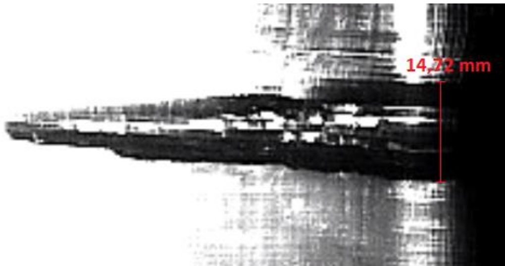
Fig. 5. The dimension of the maximum width of the temporary cavity for the first missile at a distance of 5 m.
