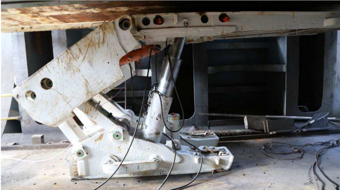
Fig. 7. JZR 13/28 POZ shield support
