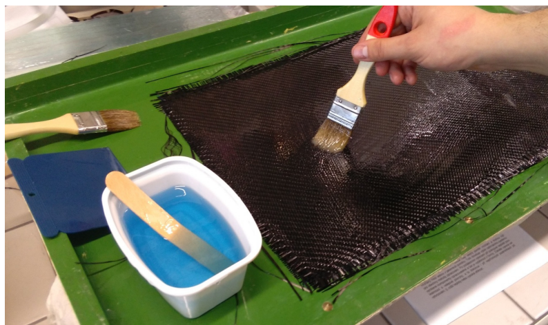
Figure 5. Production of the board by the method of manual lamination.
