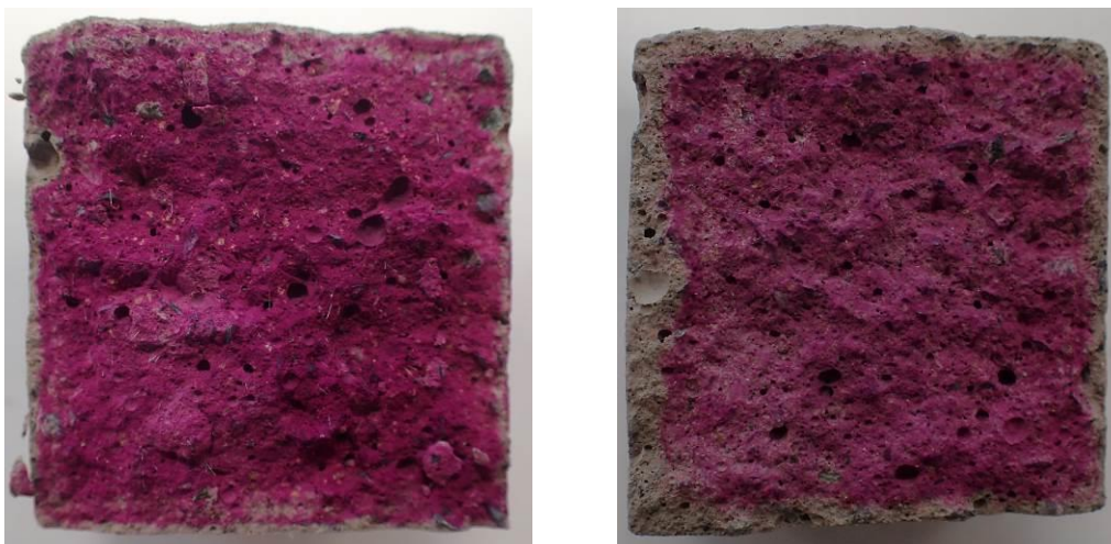
Fig. 6: Fracture area of carbonated mortar (phenolphthalein test) – 90 days (left) and 150 days (right) without high temperature exposure
