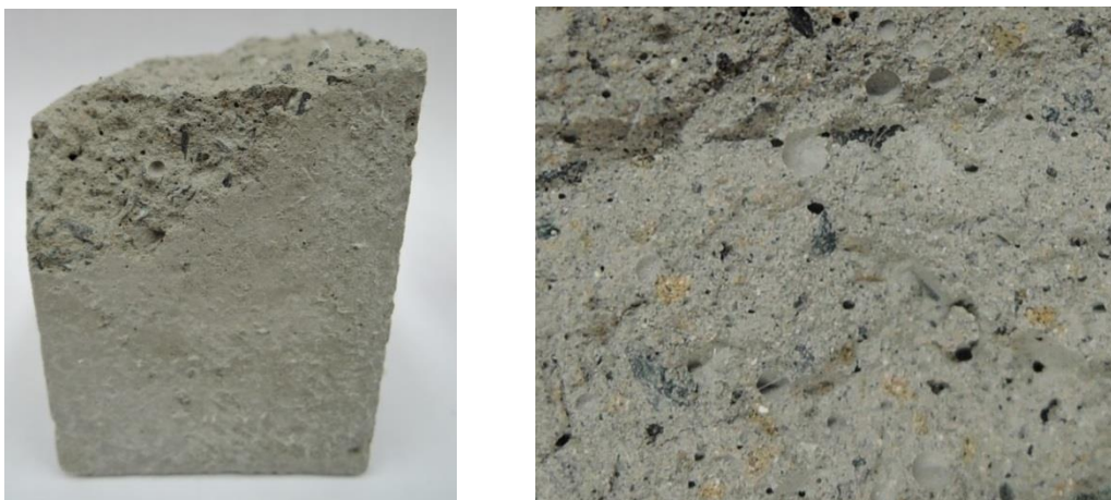
Fig.4: Sample of composite exposed in environment with increased concentration of CO 2 after 150 days without thermal stress (in graphs marked as "150-C") – surface (left) and detail of fracture area (right)
