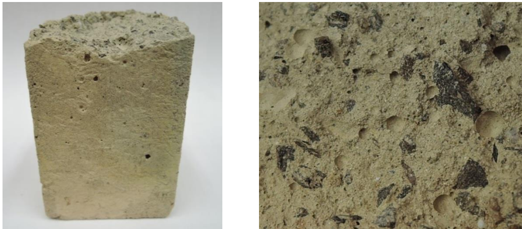
Fig. 5: Sample of composite exposed in environment with increased concentration of CO 2 after 150 days and subsequent exposition to 1,000 °C (in graphs marked as “150-C”) – surface (left) and detail of fracture area (right)
