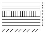
Fig. 3. Composition of sample 4A - 1,2,3,4,6,7,8,9 pre-pregs; 5 Aramid honeycomb.
