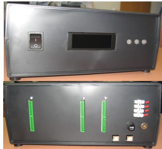
Fig. 12. The appearance of the second (new, herein described) evolution of the module – the front (up) and the back side (down).
