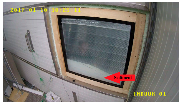
Figure 8. The sediment inside the PCM window panel.
