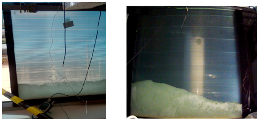
Figure 5. The melting process of the PCM glass panel, the picture on the left shows first melting process. The picture on the right shows second melting process of the PCM window panel in the calorimetric chamber.
