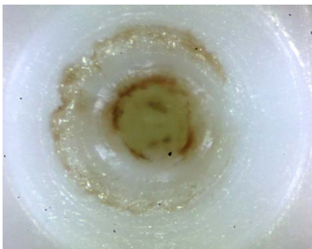
Figure 5. 100 times magnified indentation mark into irradiated PBT by 132 kGy after 5 seconds of penetration at 350 °C.
