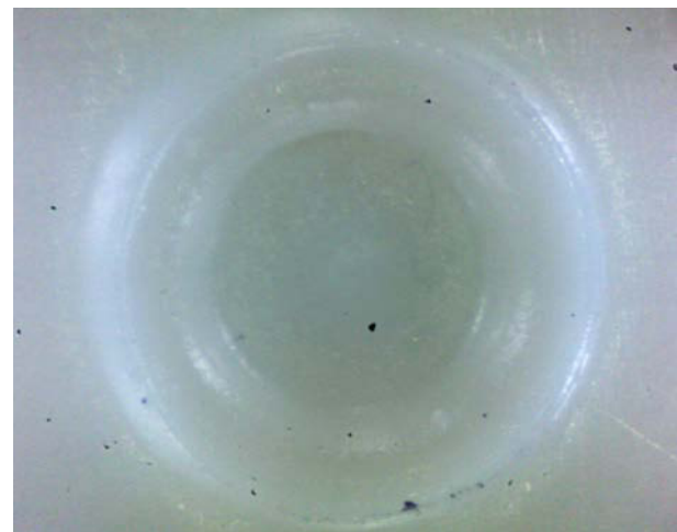
Figure 3. 100 times magnified indentation mark into irradiated PBT by 132 kGy after 5 seconds of penetration at 250 °C.
