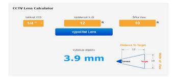
Figure 2. CCTV Lens calculator [2]
