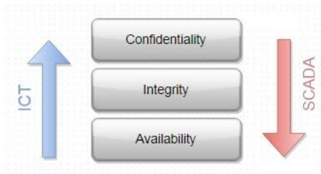
Fig. 1. The comparison of ICT and SCADA cyber security. [2]
