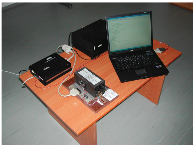
Fig. 1: Model of Hot-Air Tunnel Connected to PC via CTRL 51 Unit
