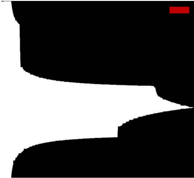
Figure 5. Mask generated from the polar image in figure 4(b) using a closing morphological operation. The bar size for the horizontal direction is 1 mm.
