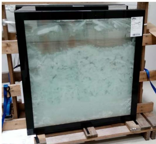
Fig. 2. Quadruple glazing panel filled with PCM.
