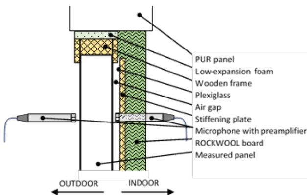
Fig. 4. Schematic representation of microphone mounts with rear-side absorption.
