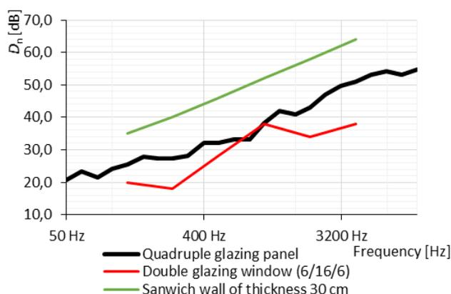
Fig. 6. Comparison of normalized difference in sound pressure levels of three types of building elements.
