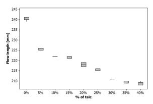
Figure 11. Influence of the flow length on filler amount (Rough design plate).
