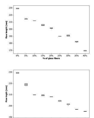
Figure 8. Influence of the flow length on filler amount (Grinded plate).
