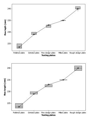
**Figure 4.** Influence of the flow length on surface quality (0% - GF top, talc bottom).
