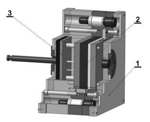
Figure 2. Assembly of injection mold.
