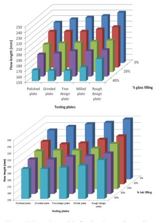
Figure 12. Dependence of the flow length on surface quality and filler amount.
