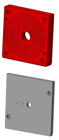
Figure 3. Cavity plate – spiral shaping plate (top), testing plate (bottom).
