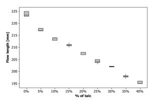
Figure 7. Influence of the flow length on filler amount (Polished plate)
