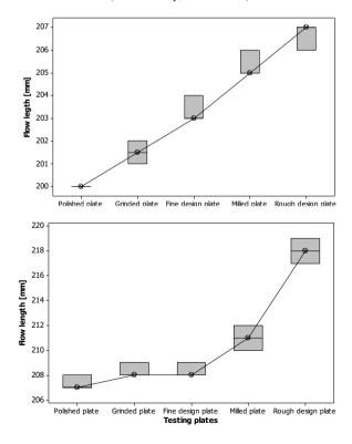
Figure 5. Influence of the flow length on surface quality (20% - GF top, talc bottom).
