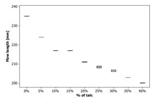
Figure 10. Influence of the flow length on filler amount (Milled plate).
