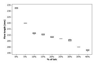
Figure 9. Influence of the flow length on filler amount (Fine design plate)
