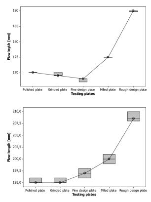
**Figure 6.** Influence of the flow length on surface quality (40% - GF top, talc bottom).
