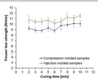
Figure 9. Trouser tear strength vs. curing time
