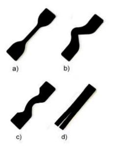
**Figure 2.** Test samples: a) dumbbell (type 1); b) crescent; b) graves; d) trouser
