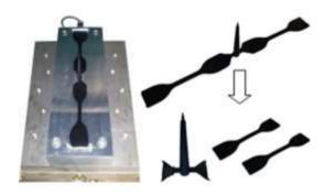
Figure 3. Production of testing samples by injection molding
