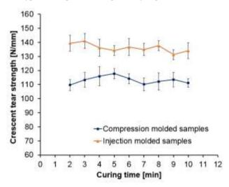
Figure 8. Crescent tear strength vs. curing time
