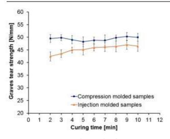
Figure 7. Graves tear strength vs. curing time
