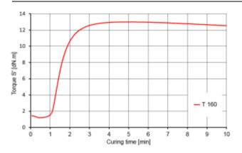
Figure 1. Curing curve for 160 °C
