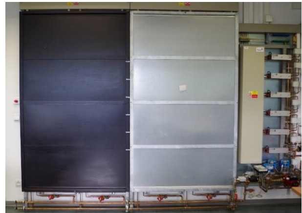
Figure 3. Thermal panels with the original and modified surfaces.
